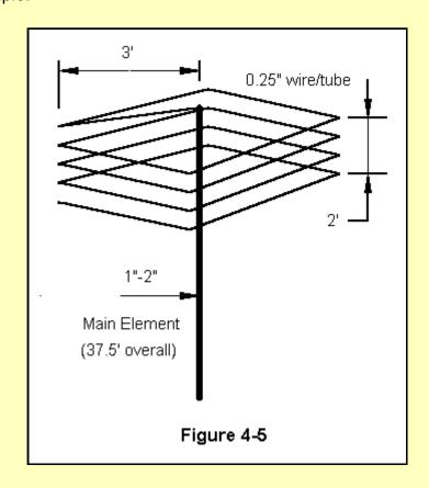
For test purposes, models were constructed using a square helix form, with each turn held at the same level and only the last of the 4 wires in the turn dropped to the next lower level. turns were spaced 0.5' apart. In the model table, the length of the coil is indicated by the number of turns and can be converted into feet by dividing by 2. Since spacing is a standard 3' from the coil, the last pair of numbers in the file name indicates the wire
