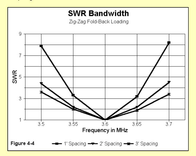
Although the 2' spaced assemblies exhibit a bandwidth similar to that of the 3' spaced top linear load, the 3' spaced zigzag assemblies show a clearly superior operating bandwidth. Added to the higher feedpoint impedance, this structure may be worth considering, despite its greater mechanical difficulties.
