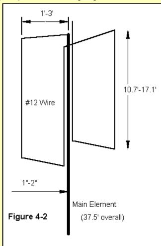
In principle, the zigzag assembly should result in a shorter overlap than the single linear top load. As a result, the antenna should exhibit additional gain, although this figure might well be marginal from an operational perspective.
