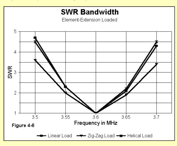
Using lossless wire against perfect ground permits a detailed comparison of the theoretical possibilities of element extension top loading. However, it is also fair to ask to what degree the use of real materials will moderate the promise shown by some of these models. The answer to
